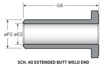
SCH. 40 EXTENDED BUTT WELD END 73E00/83E00
