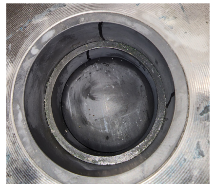
After 3 years in service, inspection of the S19L showed no signs of erosion on the ball segment, seat, body walls, or liner.
