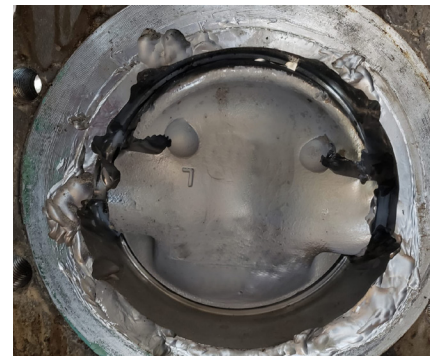
The existing ball and butterfly valves were experiencing severe erosion and leaks and jamming issues from seized valves
