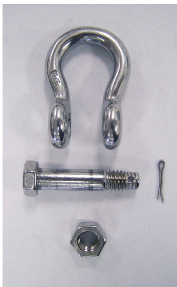
Figure 3: Anchor Shackle connected to the chain guide and Anchor Shackle Assembly.
