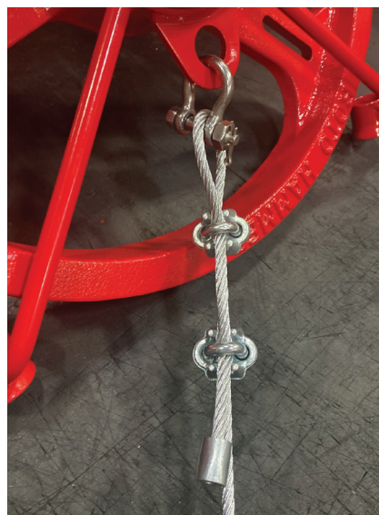
Figure 3: Anchor Shackle connected to the chain guide and Anchor Shackle Assembly.
