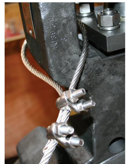
Figure 4: Wire rope secured around the neck of the valve.
