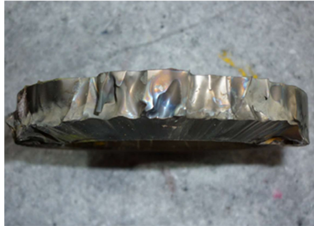
Erosion due to high velocity flow
